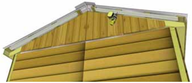
Facia/Roof Nailing Strips (4 @ 3/4" x 2 1/2" x 48"
